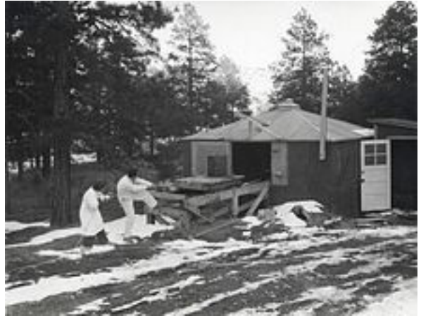
Remote handling of a kilocurie source of radiolanthanum for a RaLa (Radioactive Lanthanum) Experiment at Los Alamos.
